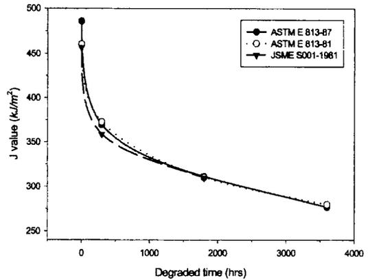
**Fig. 9** Relationship between the ASTM E 813-87, the ASTM E 813-81, and the JSME S 001-1981 SZW method for the  $J_{IC}$
