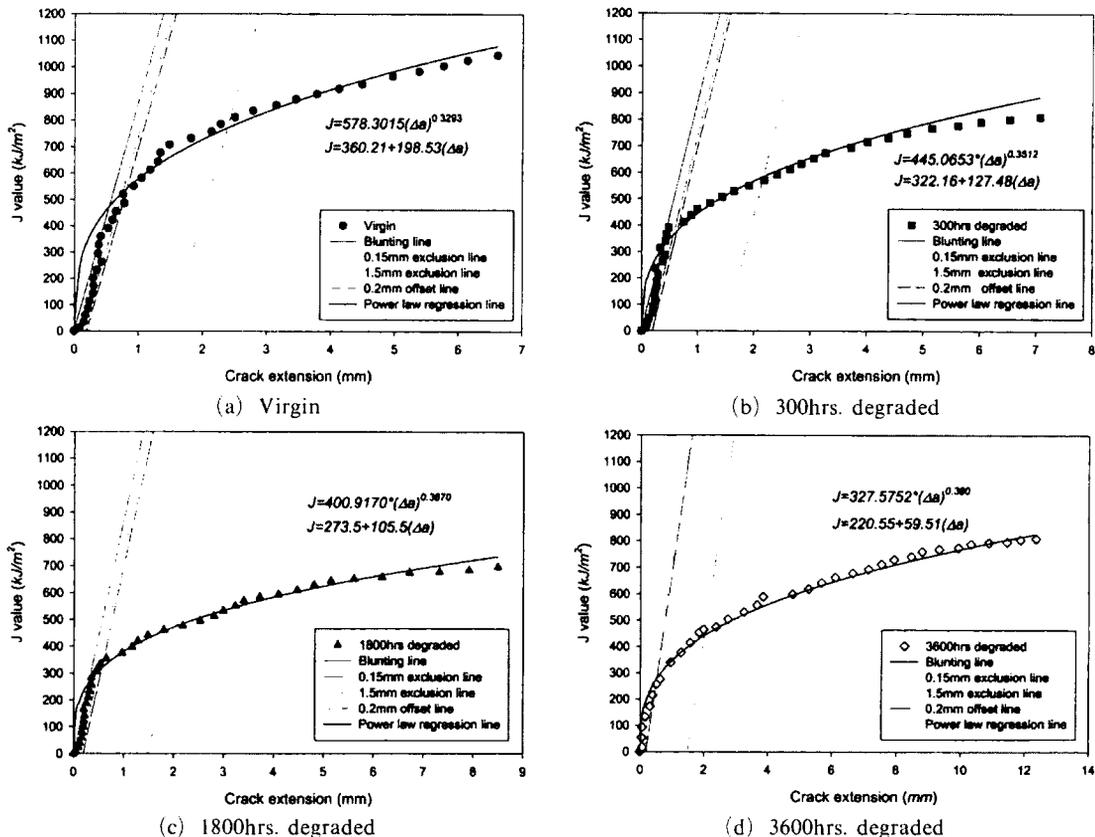
Fig. 4 Determination of  $J_{IC}$  by the ASTM E 813-87 method
