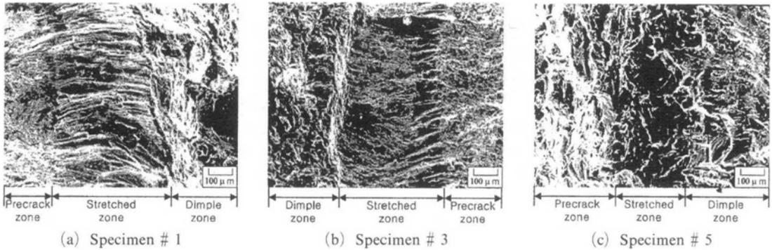
Fig. 5 Fractograph of the virgin specimens in the stretched zone
