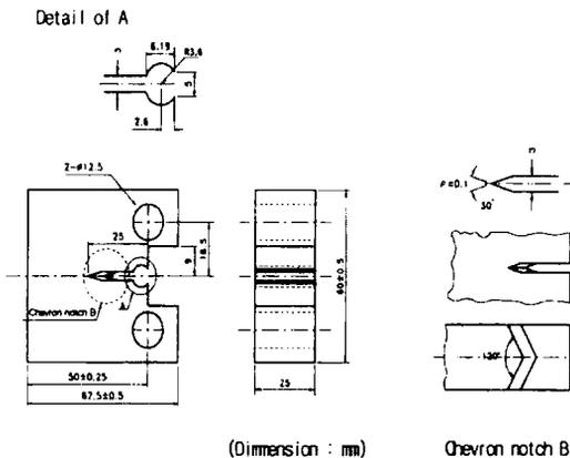
Fig. 1 Geometry of the CT specimen
